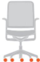
**| E |** Castors: Wrongly installed castors will affect your safety and may also damage the flooring. «Hard» castors are intended for carpeted floors, and «soft» castors are for wood or plastic surfaces. The castors are marked differently to help you distinguish them. «Hard» castors are plain coloured, «soft» castors can be recognised by the coloured contact surface, and static-conducting castors are identified by a «flash of lightning».
